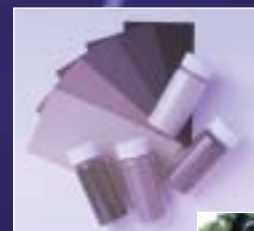
Urethane beads and the skin material made of them
