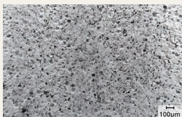
Photo 4 Electron photomicrograph of a cross section of "SANMODUR TW-E" (improved product) that was cut with a ball end mill
