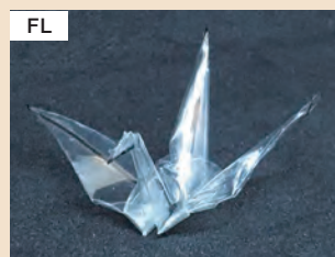
An origami crane made of a sheet which is a cured product of NEOJET FL →Because of the high toughness of cured product, cracks, etc. do not occur.
